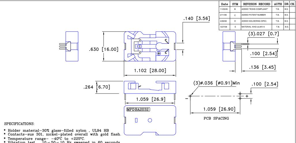
\* Vibration test  $10 \sim 50 \sim 10$  Hz sweeped in 60 seconds X,Y,Z direction 1 hour each direction Result: No dislodgement of the cell or damage No discontinuity over 10 micro-seconds.
